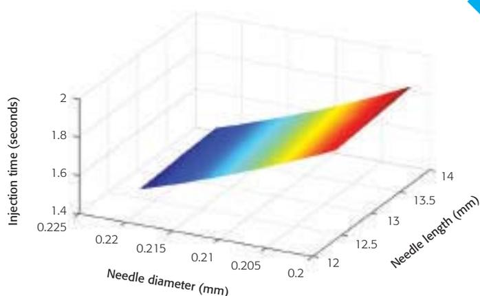
Figure 4: Injection time sensitivities to needle tolerances
