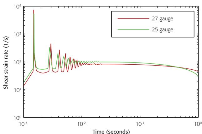
Figure 3: Drug shear strain rate predictions
