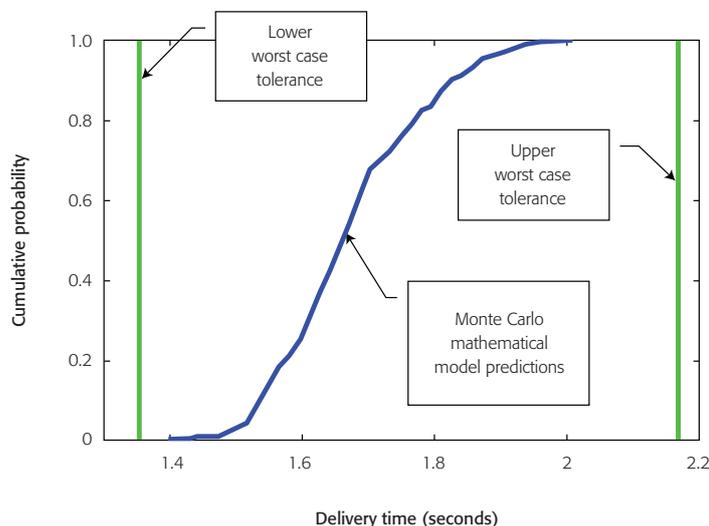
injection time results from changing the needle diameter by only -5 per cent to +5 per cent of nominal. This knowledge allows the designer to focus on the needle diameter as the single most powerful design parameter that can be used to adjust injection time.
