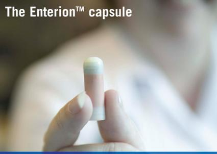
The capsule is a remote-controlled drug delivery device which delivers any form of a drug to targeted regions of the human GI tract. A gamma-emitting radionuclide sealed inside the tracer port of the capsule enables it to be tracked in real-time as it passes through the gut.
