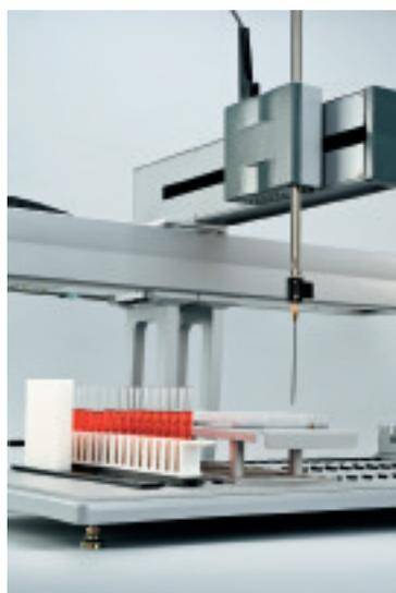
**Figure 4:** Compact modular platforms like the Tecan Cavro® Omni Robot offer a cost-effective solution for application automation
